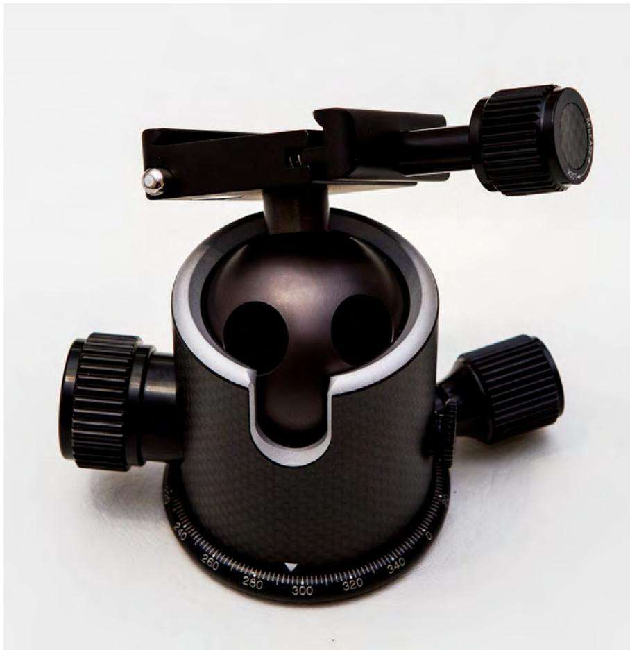
The carbon fibre construction is impressive. The locking mechanism is based on dual calipers. One dual caliper is used to lock the ball while the other is used to lock the base plate. Each caliper is operated by a rotating knob. A third flatter knob is used to maintain tension on the ball preventing any accidental flopping of mounted equipment.
